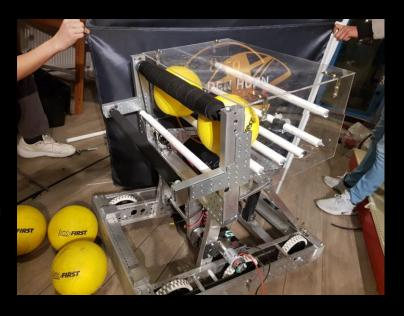
the shaft. We cut the boats of different sizes, which we bought for use in climbing up to the size, fixing small wheels to their ends and passing the rope over the wheels, and attached the end of the rope to the shaft of the PG71 engine. We fixed the hook to the end of the uppermost pipe. For design we used the following materials:
