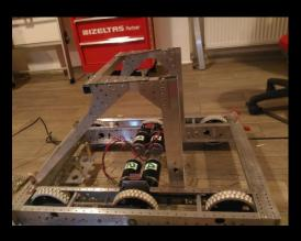
In the design of the robot, we gave the parts we have designed and we have purchased from the industry, to laser cutting. We assembled the parts from the laser cut and created the skeleton of the robot. After the intake part We used plexy, PVC pipe, roller, casing, churro, roles. Our first step in intake was to pass the churros through the pvc pipes, and then, after
